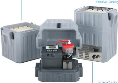
Active Cooling (autarkic temperature controlled compressor sample cooling)
